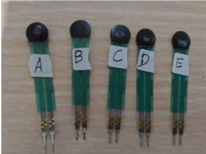
Fig. 2. The labelled FSR pressure sensors that marked their placement.
