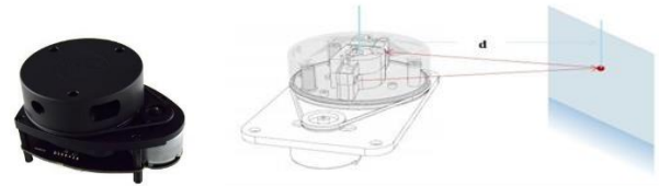
Fig.2. The LiDAR sensor (a) the physical shape; (b) The emitter and the receiver of the sensor
