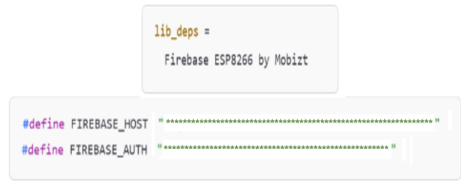
Fig. 7. Firebase software library integrated into the ESP8266 firmware for cloud communication.
