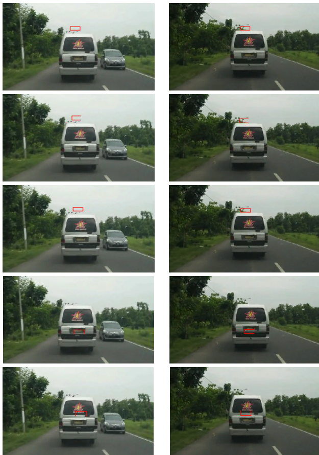
Fig. 11. Video 4 Mean Shift Tracking using (from the top) Uniform, Triangular, Epanechnikov, Gaussian and Switching Kernel. Tracking results of frames 15, 30 are displayed.
