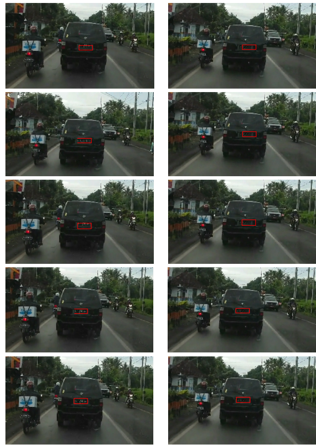
Fig. 9. Video 3 Mean Shift Tracking using (from the top) Uniform, Triangular, Epanechnikov, Gaussian and Switching Kernel. Tracking results of frames 20, 40 are displayed.
