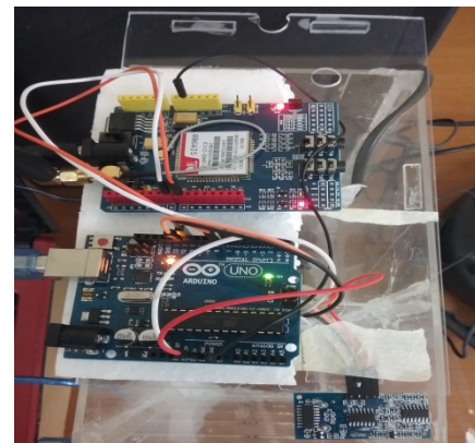
Fig. 7. Top view of the proposed flood sensor prototype.
