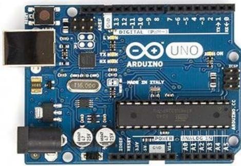
Fig. 4. Arduino UNO R3 development board [12].
