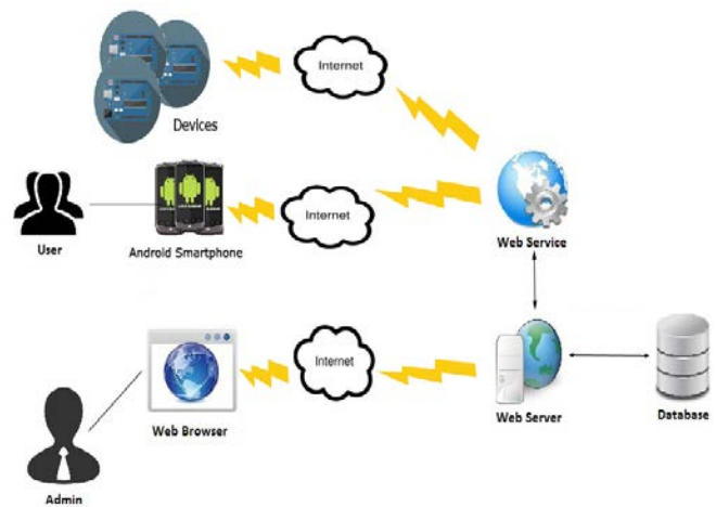
Fig. 1. Networking architecture of the telemonitoring system
