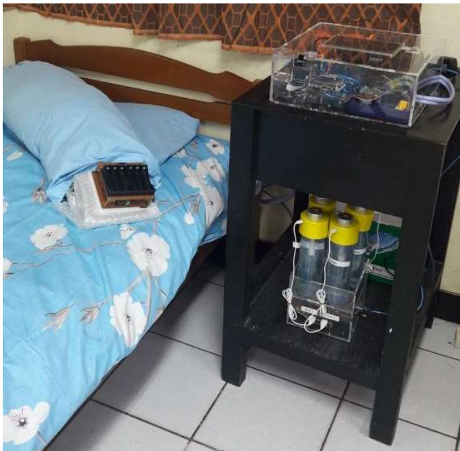
Fig. 9. The smart bed system and warm bolster. The battery module is put inside the bolster as shown in the left side while the other modules are on the black table.
