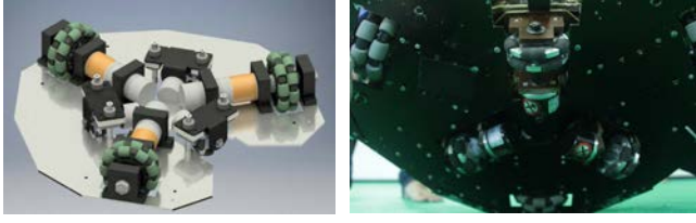
Fig. 1. Design (left) and Implementation (right) of Modified Odometry Sensor
