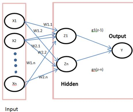
Fig 1. Architecture of Backpropagation
