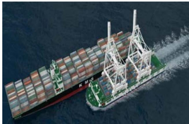
Fig. 1. A shuttle ship docking at a containership.
