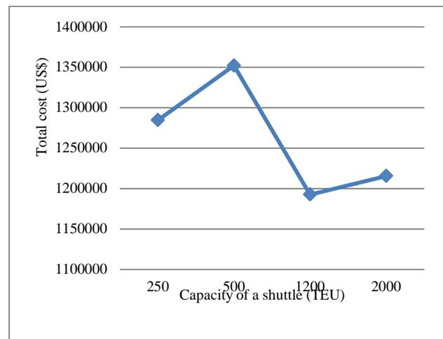
Fig. 7. The optimal shuttles capacity for the given cargo.
