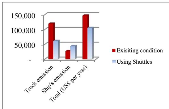
Fig. 6. The reduction of CO<sub>2</sub> emission by utilizing the offshore port services.
