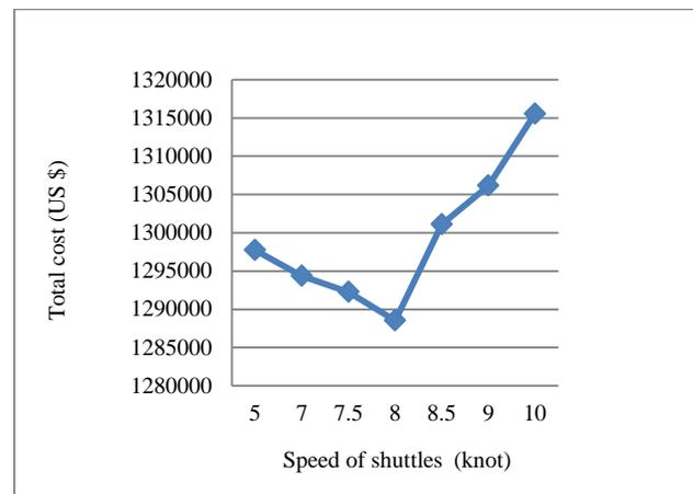
Fig. 8. The optimal speed for the given cargo
