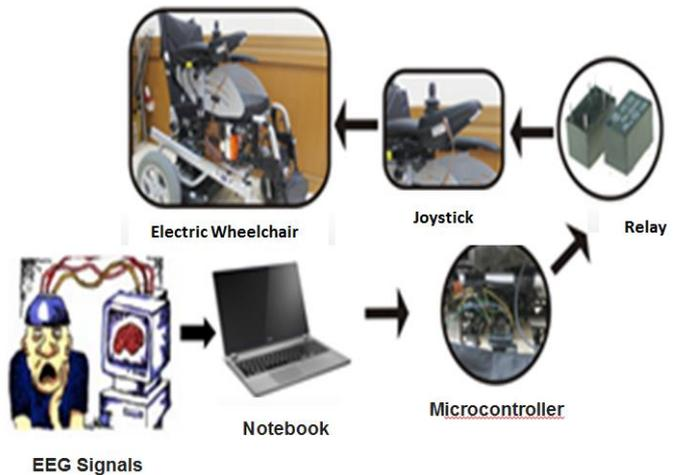
Fig. 2. Electric Wheelchair System with RS232 communication
