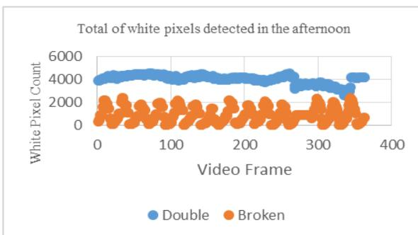
Fig. 11. Total of white pixel (lane marker) in the afternoon
