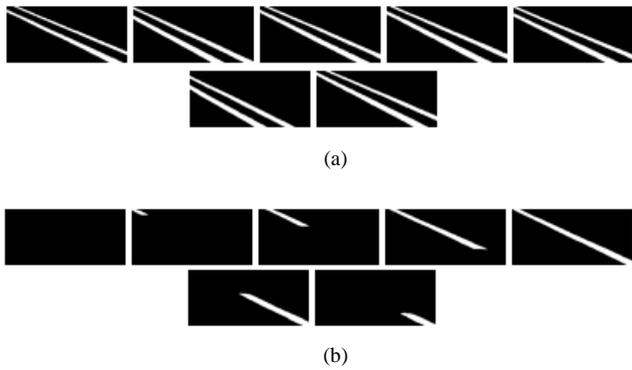
Fig. 9. The thresholding output (a) sequence of double lane (b) sequence of broken lane
