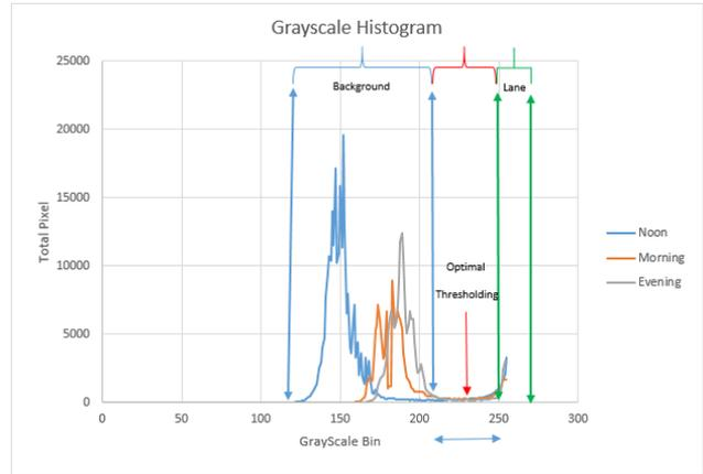
Fig. 7. Grayscale Histogram for three different time zones
