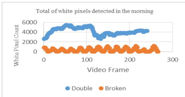
Fig. 10. Total of white pixel (lane marker) in the morning
