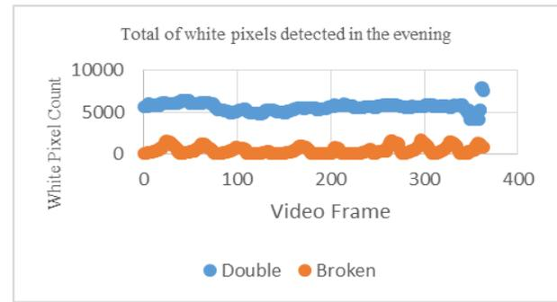
Fig. 12. Total of white pixel (lane marker) in the evening
