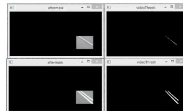
Fig. 8. The output from the thresholding process for broken and double lane markers
