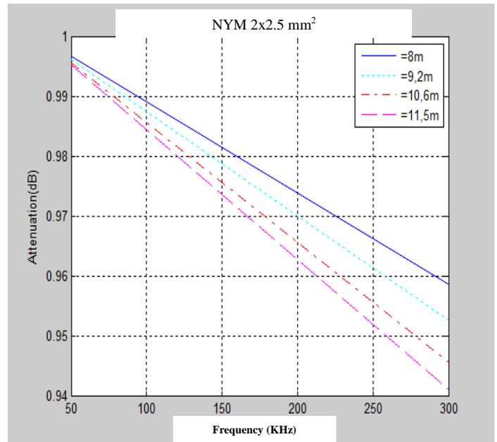
Fig. 6 The simulation results for NYM size of 2x2.5 mm² with the distance of 8m, 9.2m, 10.6m and 11.5m.
