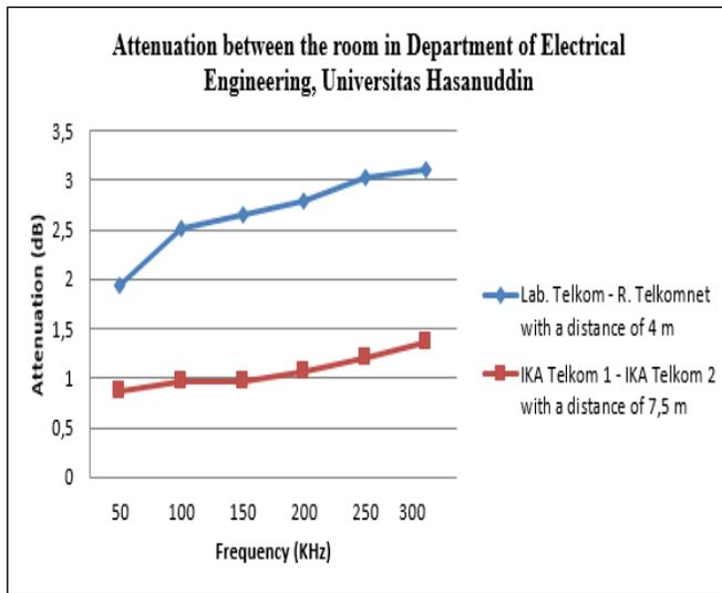
Fig. 4. Comparison of measured results between the rooms
