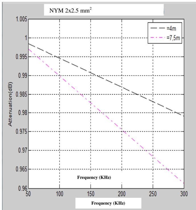
Fig. 5. The simulation results for NYM size of 2x2.5mm² with the distance of 4m and 7.5m
