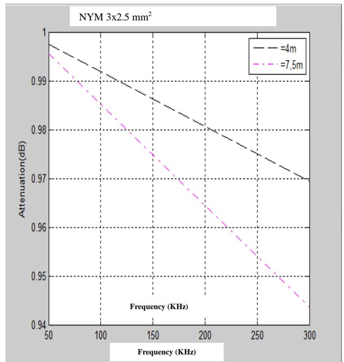
Fig. 7 The simulation results for NYM size of 3x2.5 mm² with the distance of 4m and 7.5m
