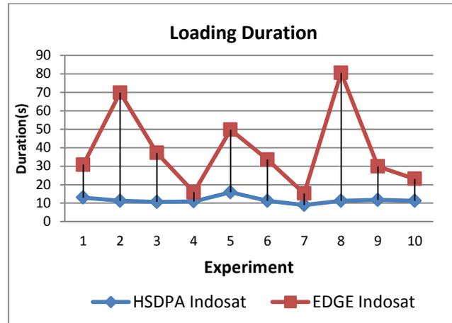
Figure 4: Loading duration against n-th Experiment Relationship.
