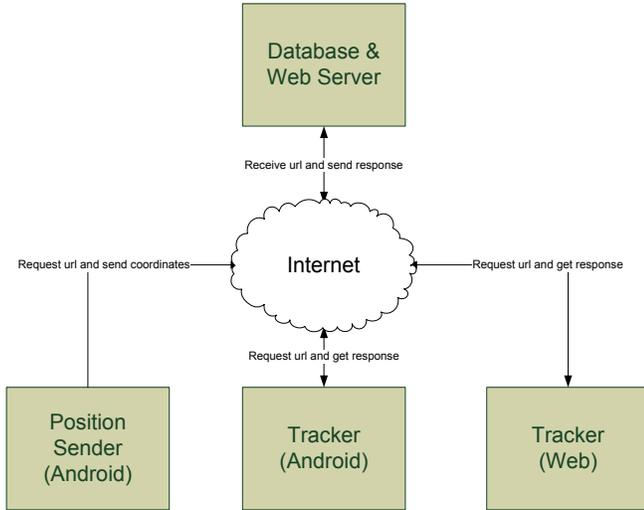
Figure 2. Diagram block of the system
