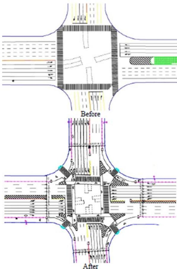
Figure 1: Intersection before and after meticulous design
